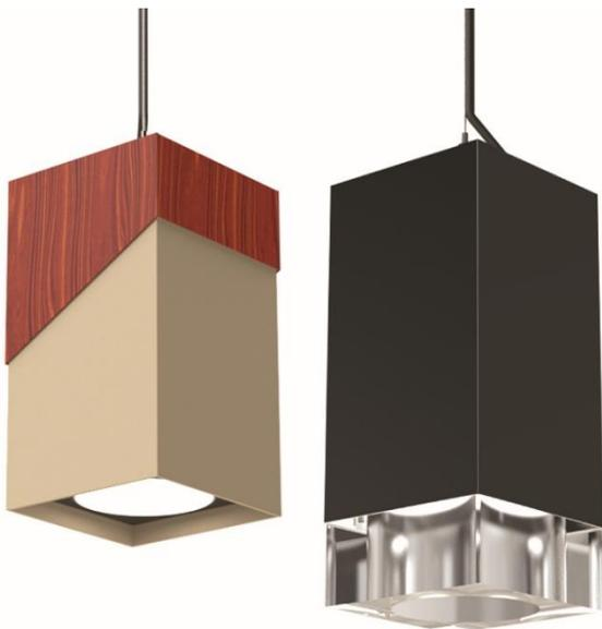
The construction of the LumiCube line is comprised of quality extruded aluminum housing and diecast components that have been designed to complement nearly any décor. With an IP65 rating, these fixtures have double gaskets at the housing apertures and the heavy UV-rated powder coat paint provides the best protection available when used in an exterior setting.
