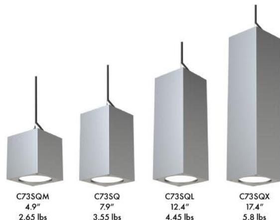
Pathway's new 4.38-inch square fixture is available in four lengths, six mounting options, three beam spreads, and up- or down-light, bi-directional, wall wash and Type II forward throw. The output of 3000 lumens (a total of 6000 lumens up/down) presents ample light for any space.
