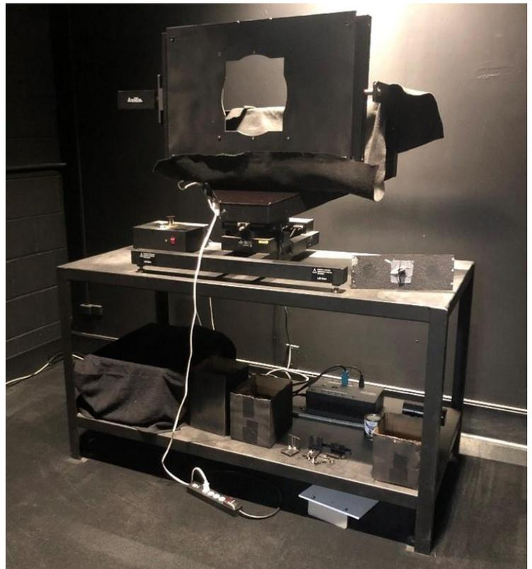
A flicker sensor was added to enable analysis of lamp flicker parameters such as those required by California's Title 24 and the NEMA 77 standard. In addition, new software enables calculating a complete set of TM-30 color rendition data as specified by a recent ANSI/IES TM-30-20 standard and making this information available to our customers.
